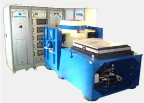
The hydrostatic bearing guidance of resin-bonded fiber reinforced armature coil takes care of cross axis even at high acceleration tests.
