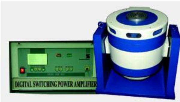
Engineering institutions and test laboratories use low thrust shakers for experimenting by injecting frequencies in a wide band.
